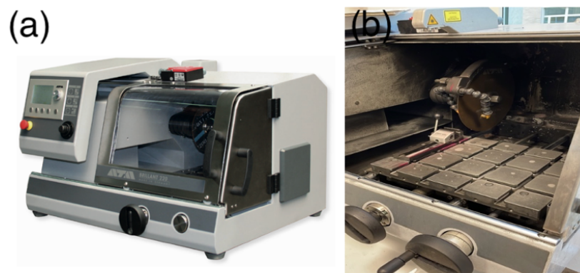
Figura 10: (a) Troncatrice ATA Brillant 220; (b) lama Cernet.
