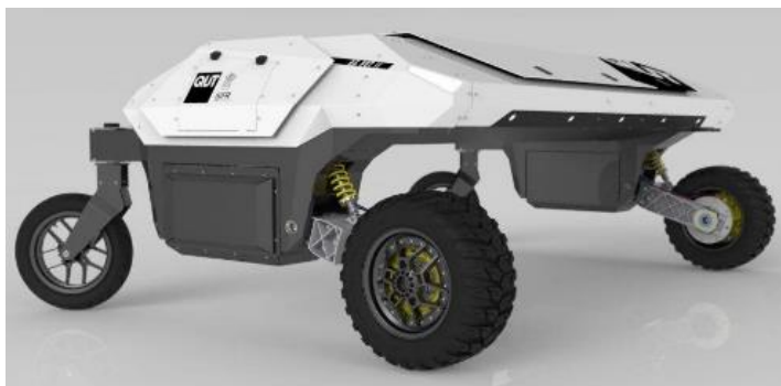
Figura 2.4 AgBot II [17] a sx, Vinerobot II [18] a dx, sospensioni passive
