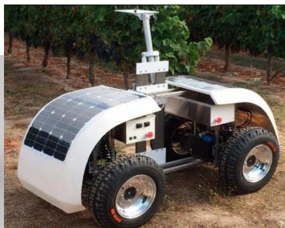
Figura 2.4 AgBot II [17] a sx, Vinerobot II [18] a dx, sospensioni passive
