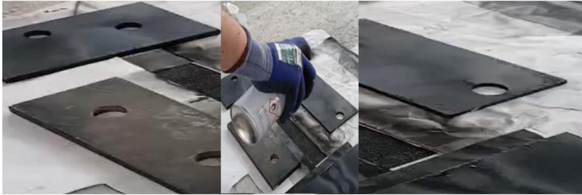
Figure 6.6 Spray application using a test stencil
