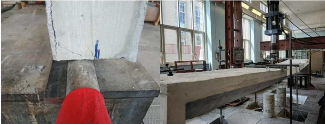
Figure 4.21 Left, sliding of the beam on supports, Right deformation at the end of the test.
