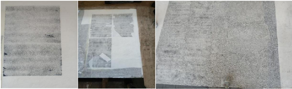
Figure 6.12 Application of the speckle pattern on the beam
