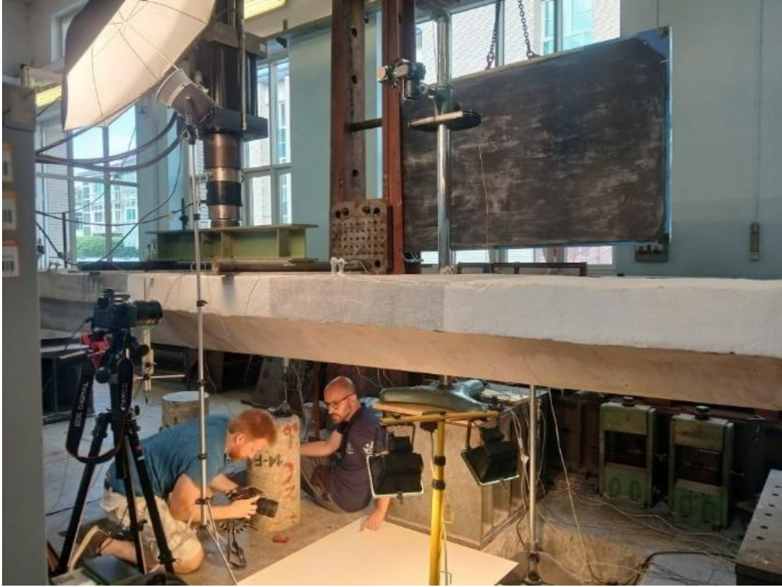
Figure 4.5 Beam preparation, test environment and installation of the camera prior to testing
