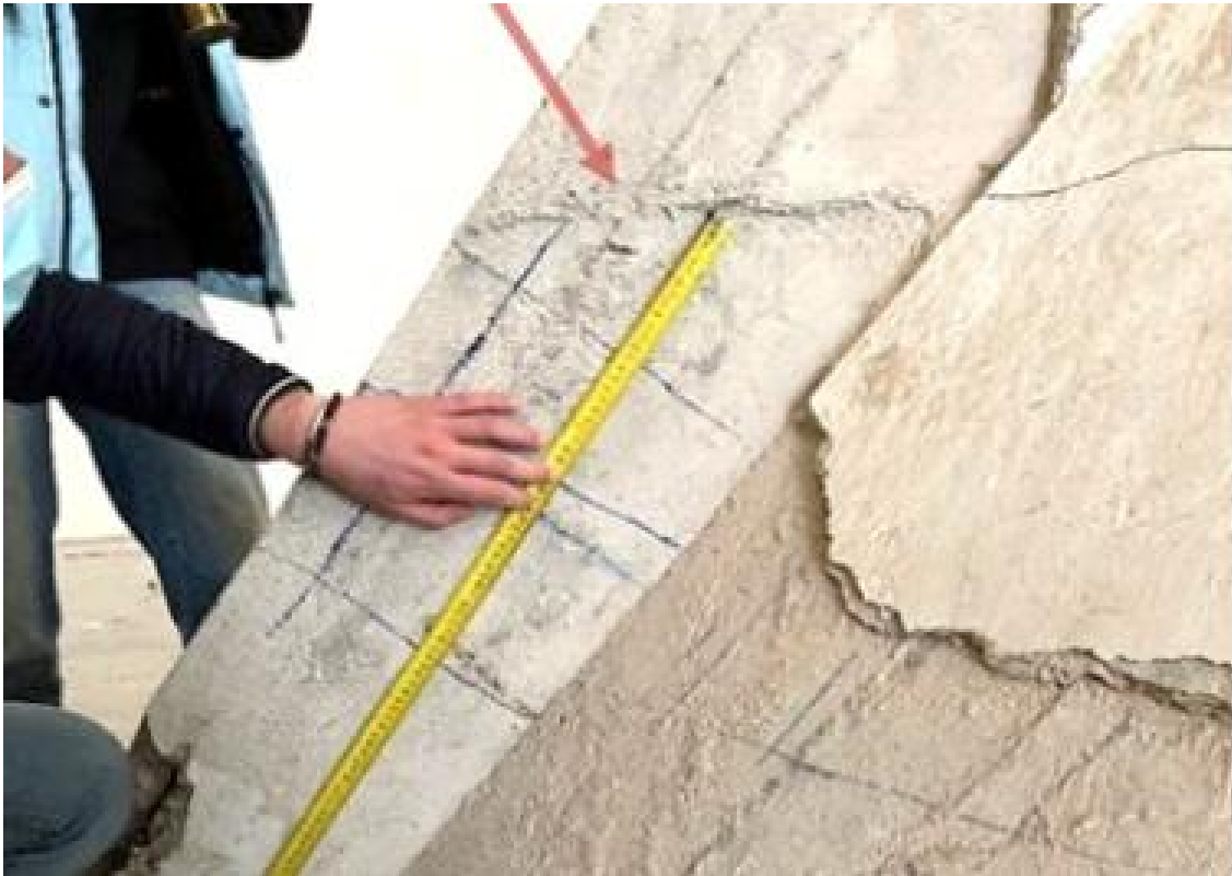
Figure 3.5 Cracking pattern observed at the base of the inclined
