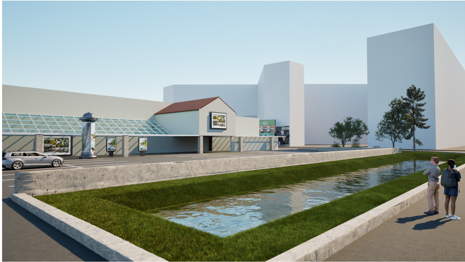
Figure 3.29: 3D model of the proposed stormwater detention system – View 1 - Close-up view [34]
