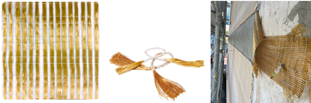
Figura 5.33: Sistema FRCM: Laterlite PBO-MESH 44 + MX-Laterlite PBO
