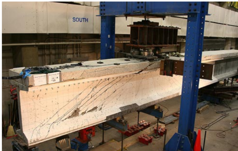
Figure 5.19: Shear testing of a 54-inch deep, LWHPG prestressed girder in the Structural Testing Laboratory at the Turner-Fairbank Highway Research Center.
