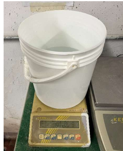
Figure 5.18 - Water weighting with the laboratory precision scale
