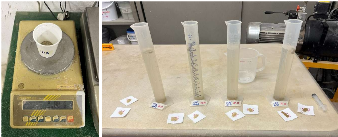
Figure 5.9 - Bentonite weighing (left) and graduate cylinder during swell index test (right)
