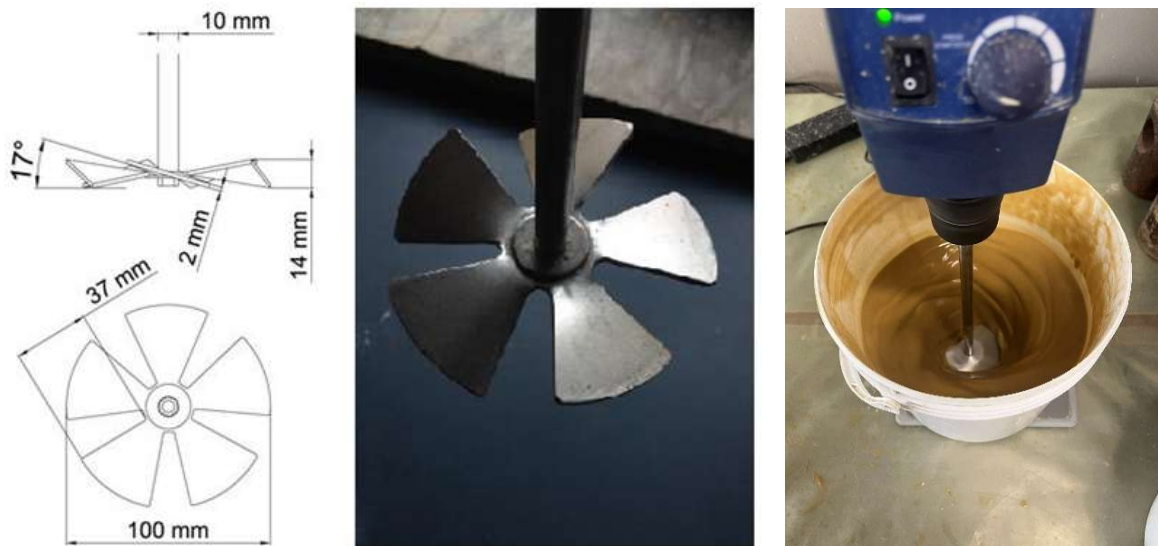
Figure 5.19 - Scheme of the used impeller (Todaro et al., 2019) (right) and photo of the utilized propeller (left)
