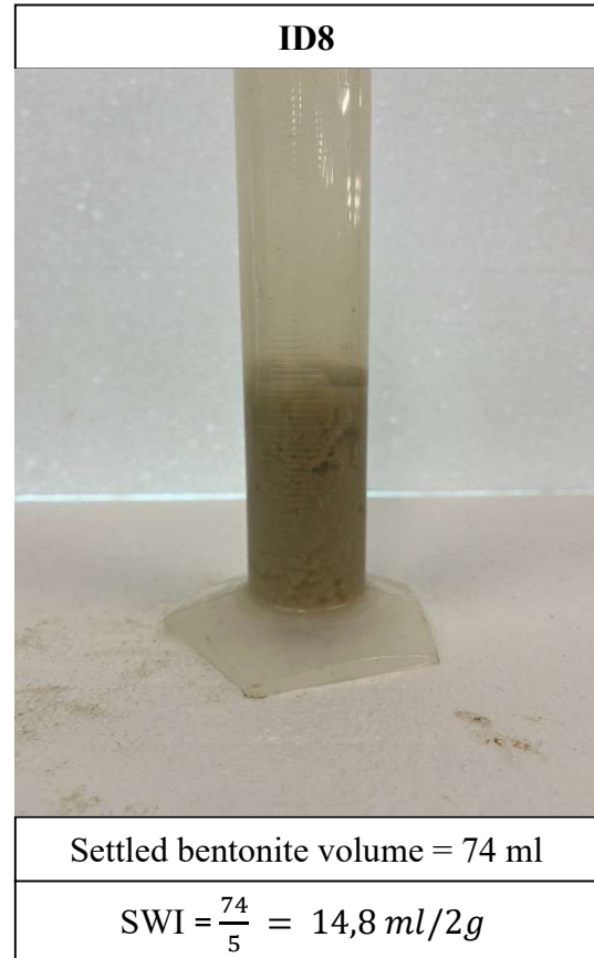
Figure 5.17 - Bentonite ID8 swell index
