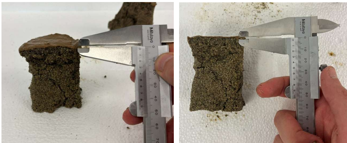
Figure 6.61 - ID7 80 kg/m 3 caliper measurement of filter cake thickness
