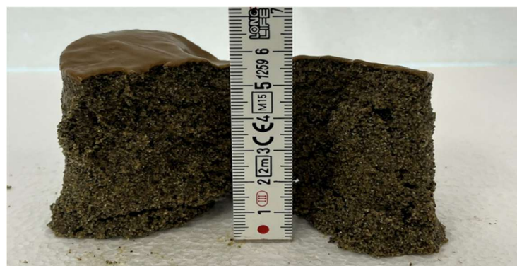
Figure 6.57 - ID7 60 kg/m 3 filter cake open and measured
