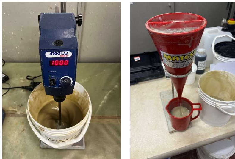
Figure 5.21 - Slurry subjected to mechanical stress (left) and immediately tested (right)
