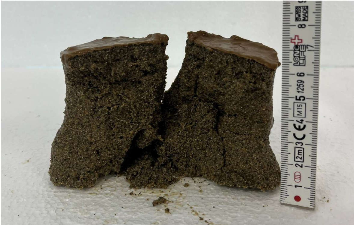
Figure 6.60 - ID7 80 kg/m 3 filter cake opened and measured
