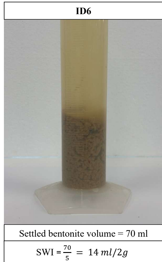
Figure 5.15 - Bentonite ID6 swell index
