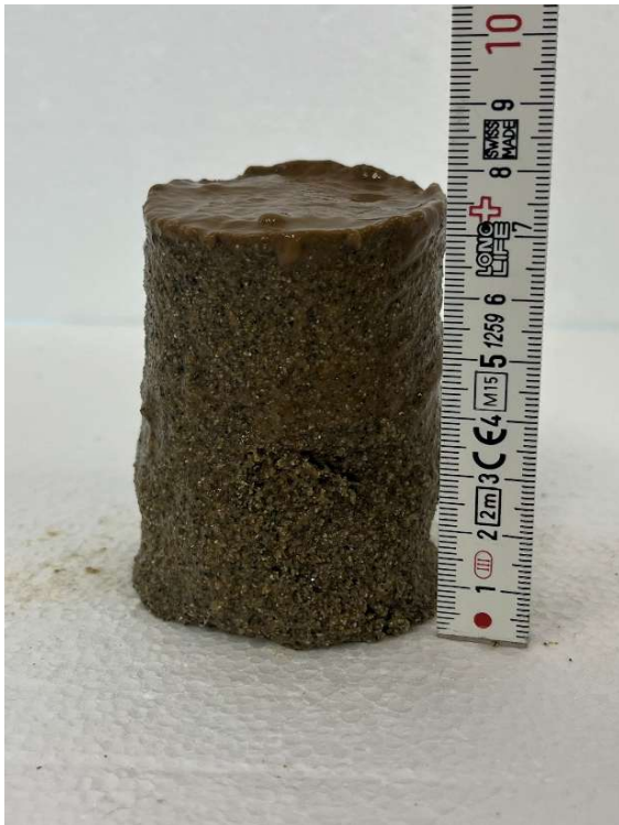
Figure 6.58 - ID7 80 kg/m 3 filter cake
