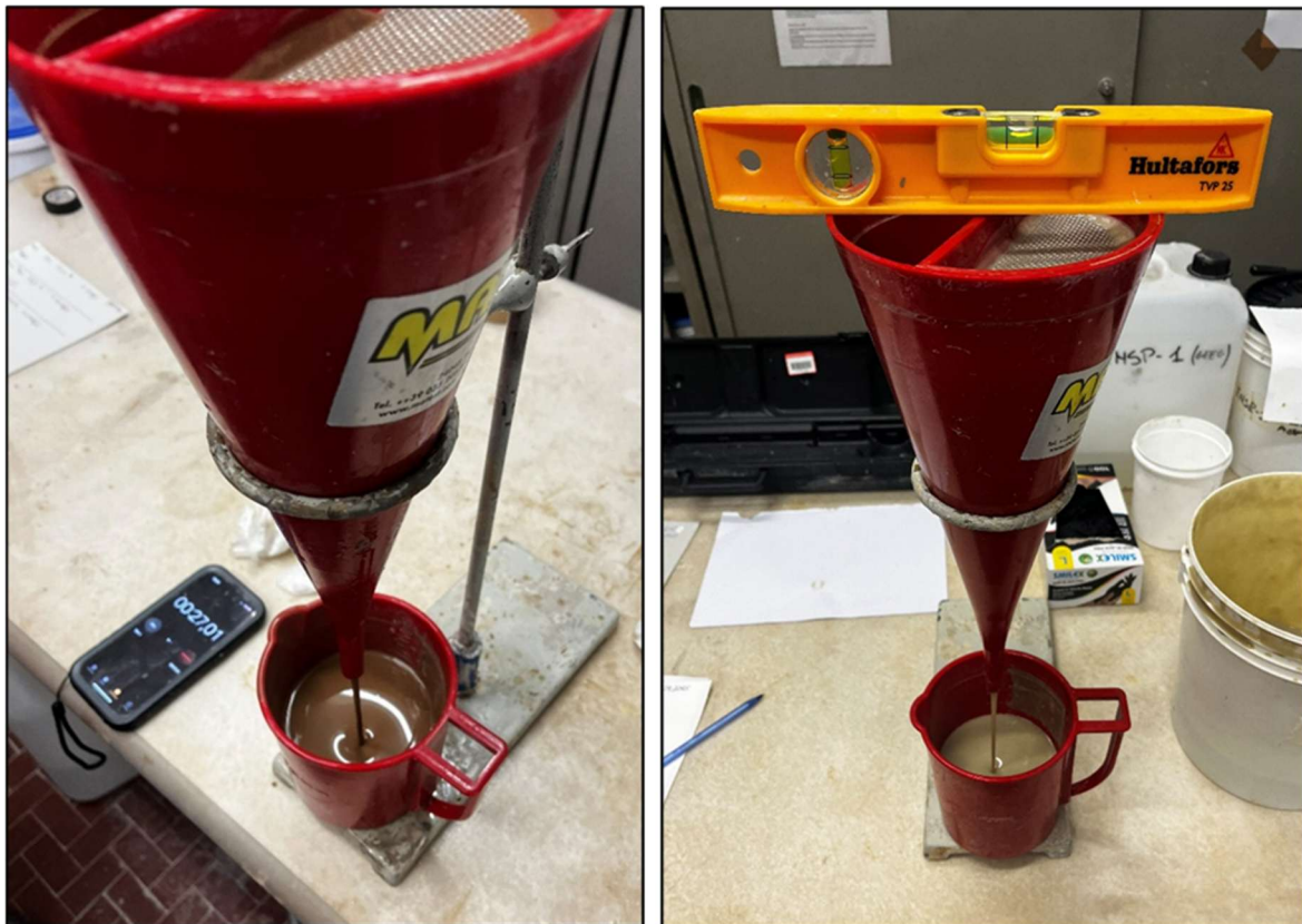
Figure 5.20 - Marsh cone apparatus and the stopwatch during test (left), checking the vertical alignment of the Marsh funnel on the metallic stand (right)
