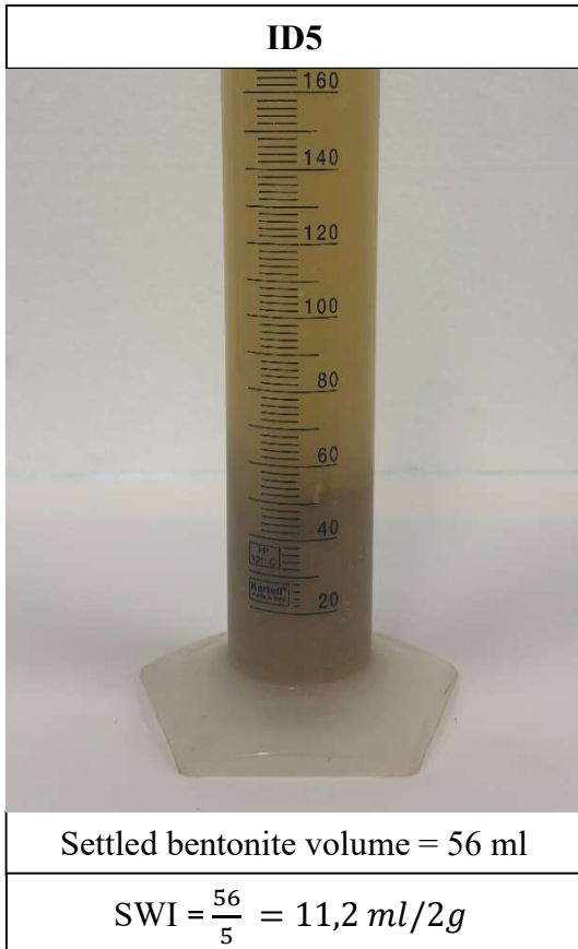
Figure 5.14 - Bentonite ID5 swell index
