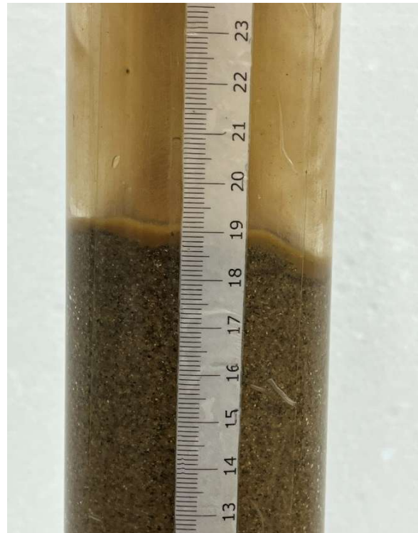
Figure 6.59 - ID7 80 kg/m 3 filter cake and slurry penetration
