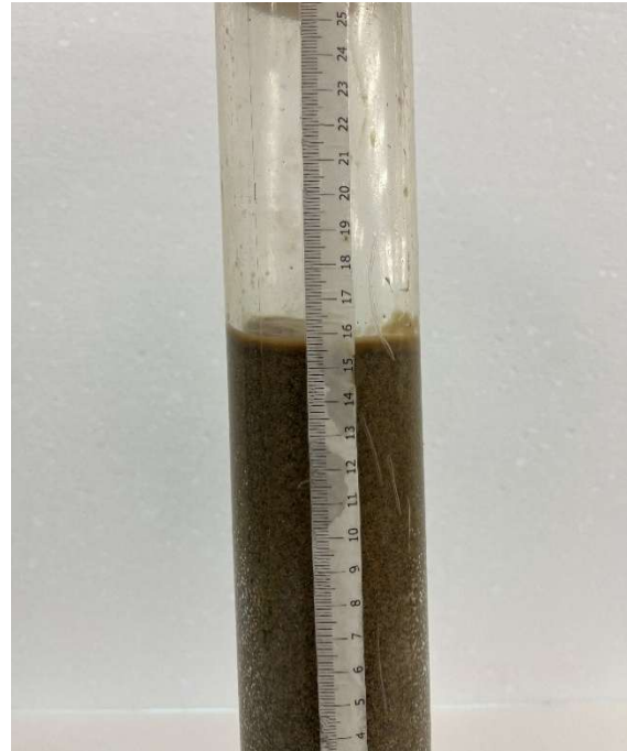
Figure 6.56 - ID7 60 kg/m 3 filter cake and slurry penetration
