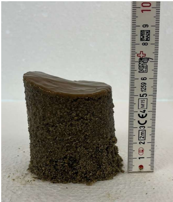
Figure 6.55 - ID7 60 kg/m 3 filter cake
