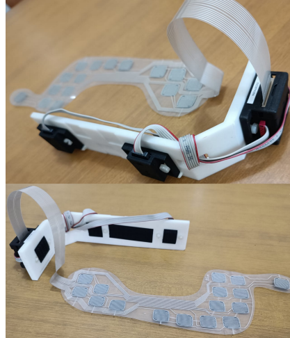
Figure 2.17: Rigid support with two distance sensor and one IMU
