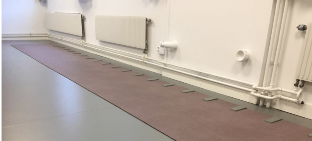
Figure 1.5: Illustration of a GaitRite pathway. Picture taken from [21]
