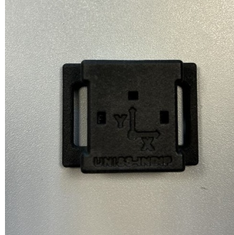
Figure 2.15: MIMU of INDIP system
