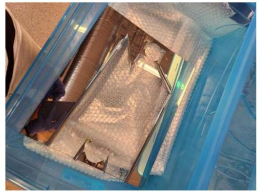
Figure 6.8: Curled up 5.5 μm Membrane
