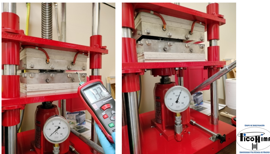
Figure 9. (9.1) Heated press for the MEA treatment at 130°C and 60 bar; (9.2) Close-up of the MEA inside the press
