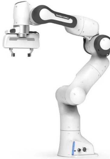
Fig. 1.2 Franka Emika Panda/FR3 collaborative arm used as the primary manipulator in this work.
