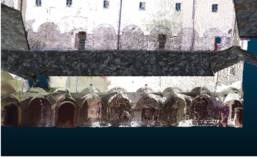
Figure 3.27: Detail of Novalesa Cloister point cloud
