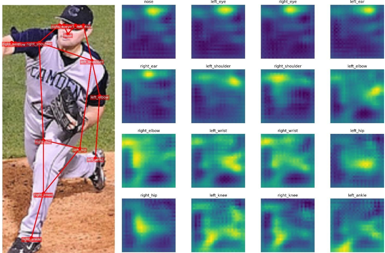
Figure 3. A visualization of the heatmap regression technique for keypoint detection. The model predicts a distinct heatmap for each keypoint (right), where the brightest area indicates the most likely location. These heatmaps are then used to determine the final keypoint coordinates on the input image (left). [40]
