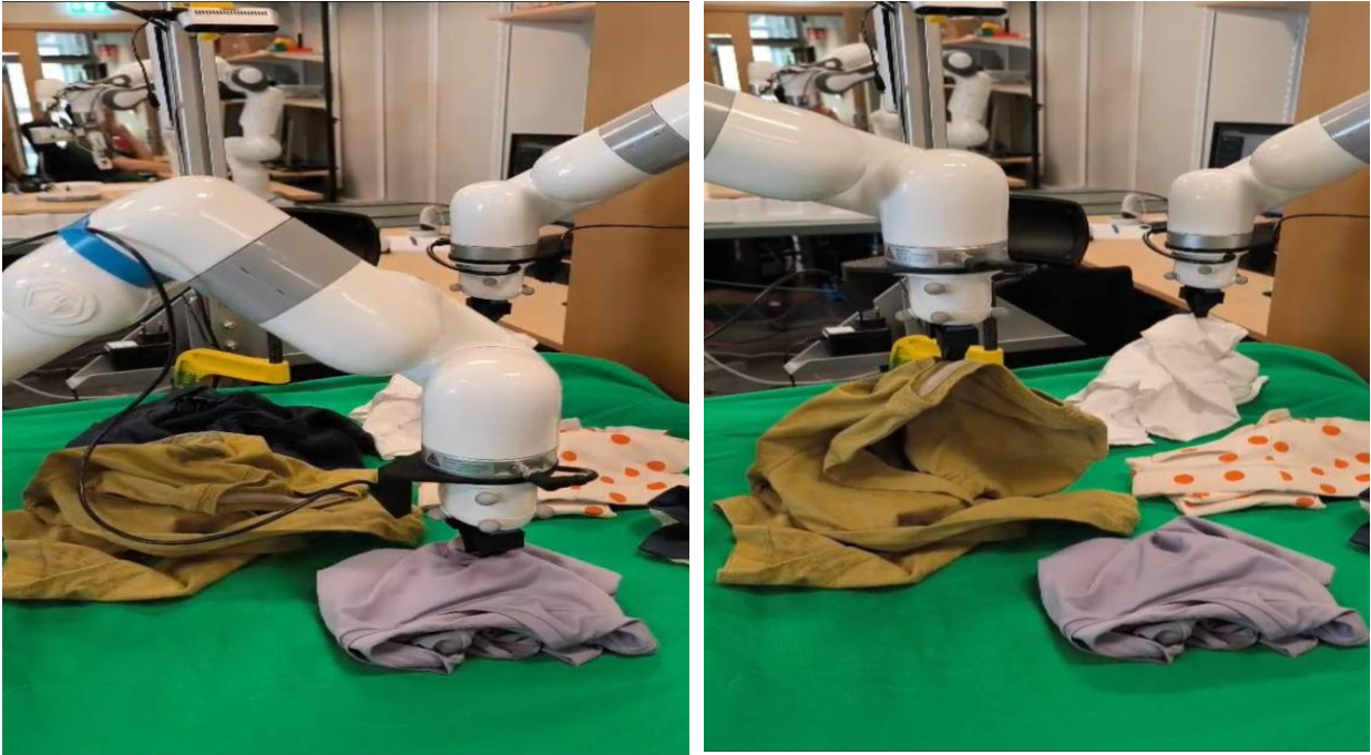
Figure 20 - instance segmentation testing with robotic arms with the Yolo v11 Nano model trained for 200 epochs. The robustness of the model is shown in real world applications.
