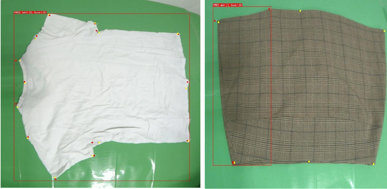
Figure 23 – (left) inference of key point detection for test 1, group 1 on a t-shirt, (right) inference of key point detection for test 7, group 4 on a skirt, the red points are the predicted ones, and the yellow points are the ground truth
