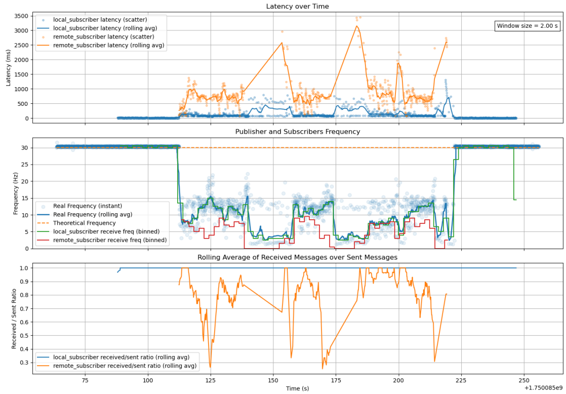
Figure 6.3. Network test conducted with ROS 2, FastDDS.
