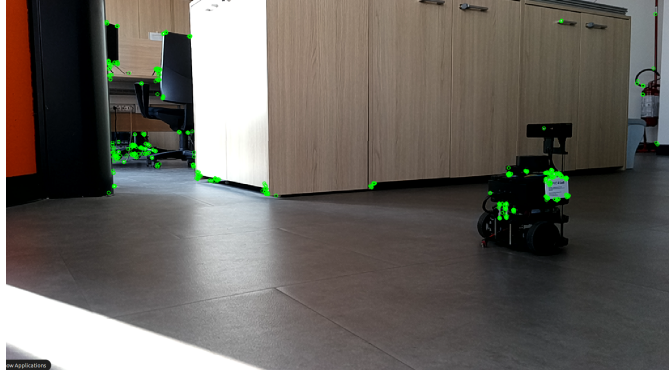
Figure 4.3: RGB-D image keypoint and feature extraction
