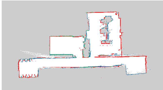
Figure 5.53: Experiment 5 - Confusion error metric (Green – TP, White – TN, Blue – FP, Red – FN)
