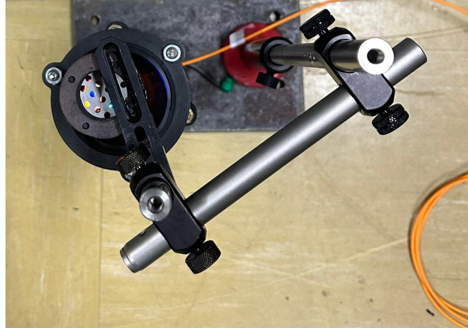
Figure 3.30: Static experimental setup to measure axial stiffness, upper view.
