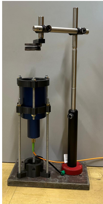
Figure 3.29: Static experimental setup to measure axial stiffness, front view.
