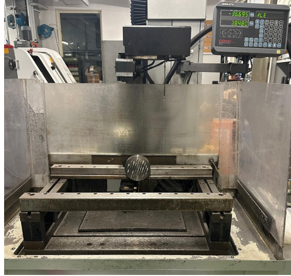
Figure 3.19: Electrical discharge machining process.
