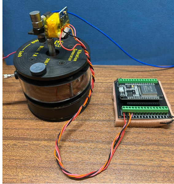
Figure 4.10: Dynamic calibration setup: vibration generator.
