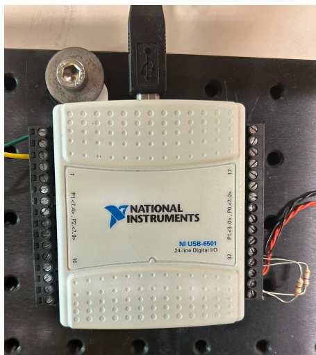
Figure 4.18: NI USB-6501 National instrument board.
