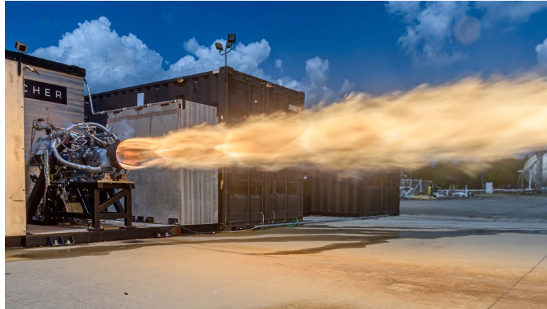
Figure 1.2: Modern liquid rocket engine test firing on small test bench (credits: launcher space/NASA)
