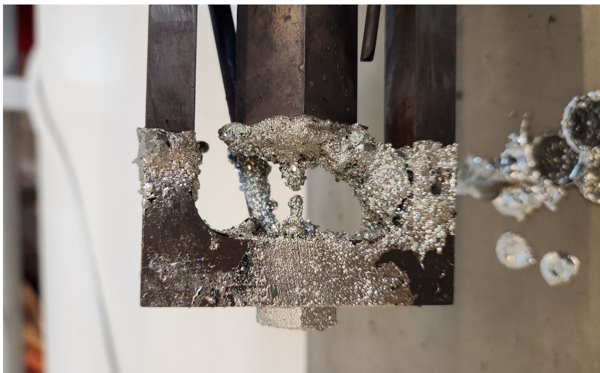
Figure 4.21: Solution precipitates observed in the area surrounding the specimen after opening the rig following the test of the notched sample in Pb+1.2 wt% Te.
