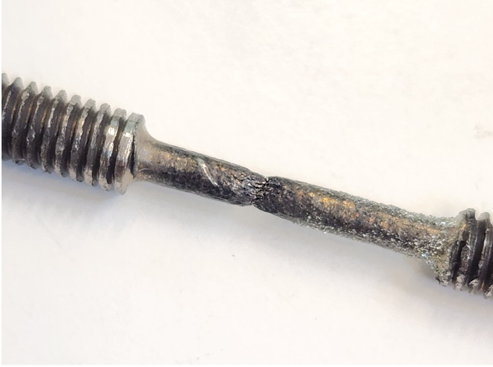
Figure A.1: Close-up of the specimen halves reassembled after the test, ready for measurement.
