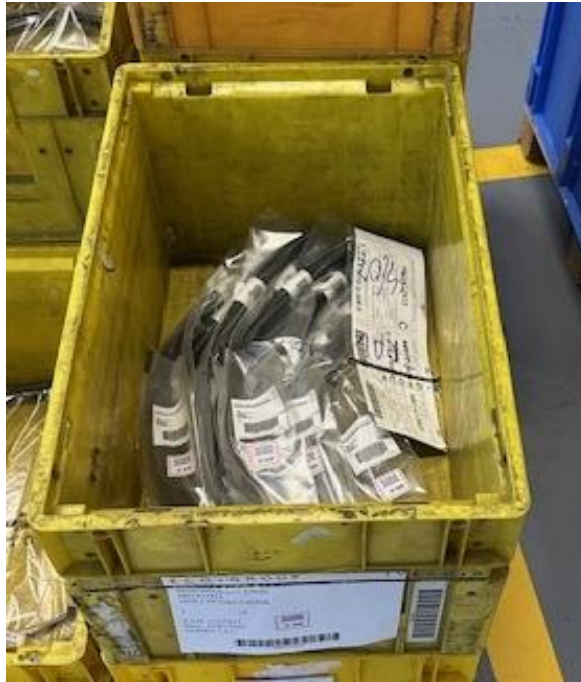
Figure 10: Odette container (DEMAC) with material to be stored
