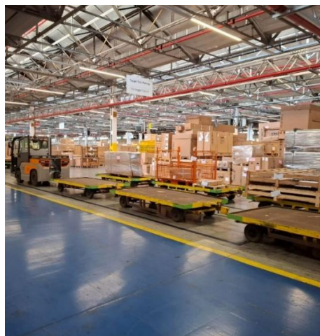
Figure 25 Tugger Train: Motor Vehicle connected to 3 Wagons
