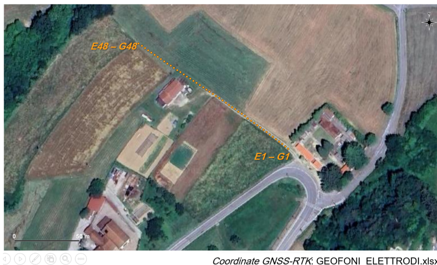
Figure 3.2. Geophone and electrode layout.
