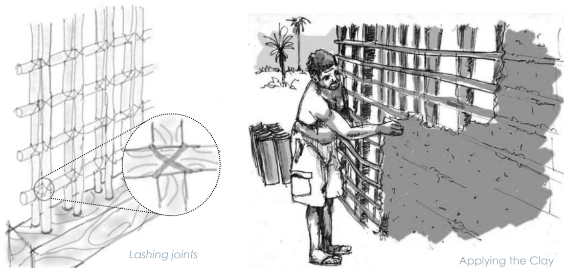
Figure 52 – Wattle and daub construction process [Source: Images from the lecture "Arquitetura Colonial Brasileira – Técnicas Construtivas," course: Theory, History and Criticism of Architecture and Urbanism II – TH2, PUC Goiás.]
