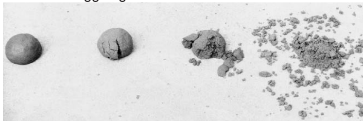
Fig. 152 Immagine del dropping test. Fonte: Minke, Gernot. Building with Earth: Design and Technology of a Sustainable Architecture. Third and revised edition. Basel, Switzerland: Birkhäuser, 2013, pag. 23
