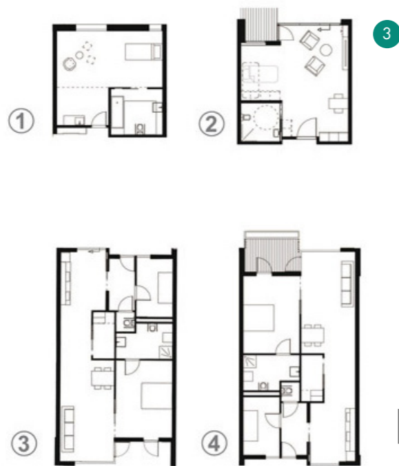
Fig. 76 Eltheto Housing & Healthcare apartment plans (Scale - 1:200). Source: 2by4 Architects (2015) - re-elaboration of the author
