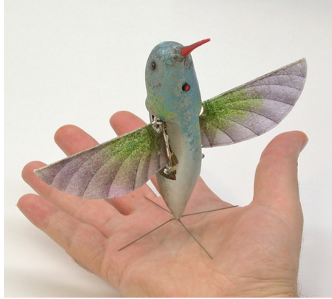
Figure 1.1: Flapping-Wing Micro Air Vehicle, from Keennon et al. [4]
