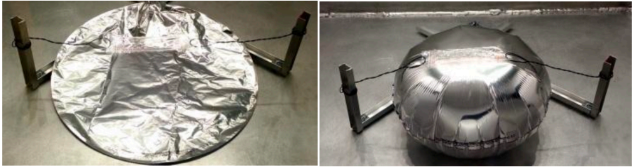
Figure 13.2 Inflation of antenna sample on left, rigidization on right [37]
