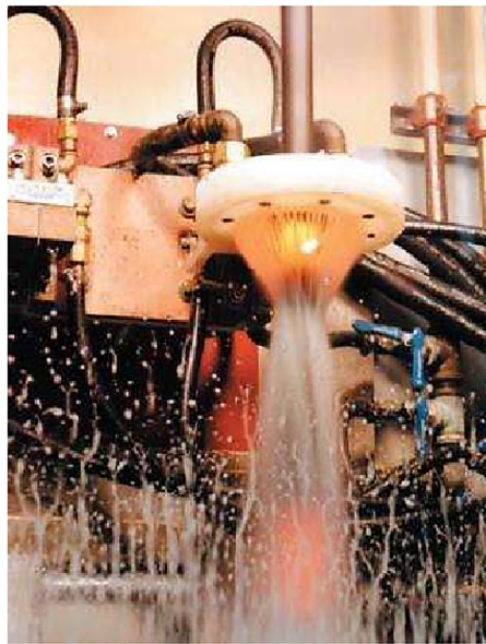
Figure 2.7: Example of the setup for spray quenching [17].
