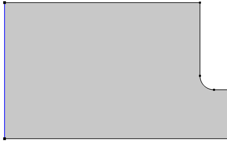
Figure 3.16: Edge where the Axial Symmetry condition has been applied.
