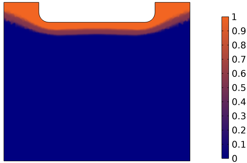
Figure A.4: Austenite distribution across the crankpin after heating.
