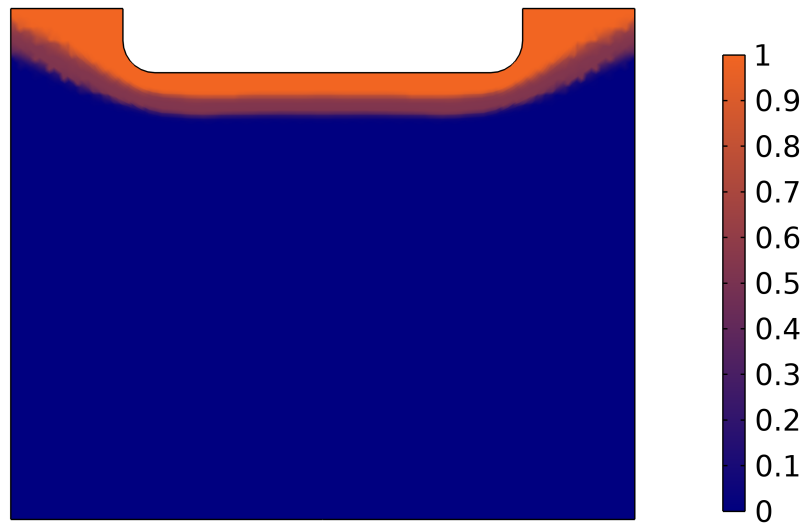
Figure 4.4: Austenite distribution across the main bearing after heating.
