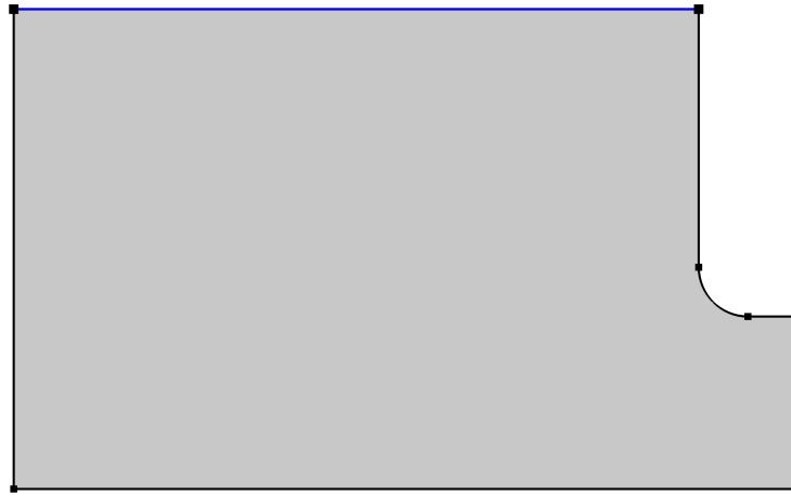
Figure 3.17: Edge where the Symmetry condition has been applied.
