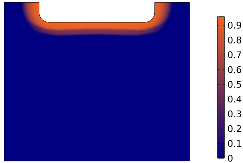
Figure A.7: Martensite distribution across the crankpin after heating.
