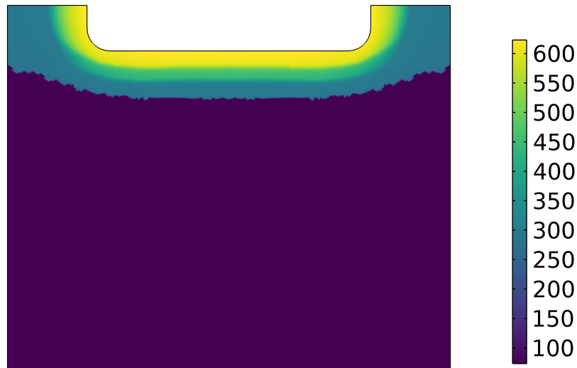
Figure 4.9: Vickers hardness profile across the main bearing.
