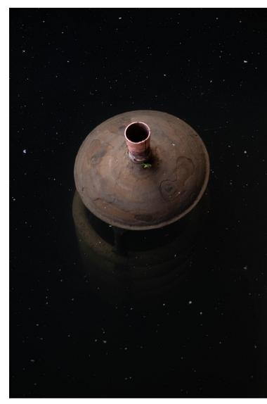
Serpentine in its cold water bath. The vapor from the boiling fermented mash travels through this copper coil that cools it down, condensing it back into liquid mezcal.
