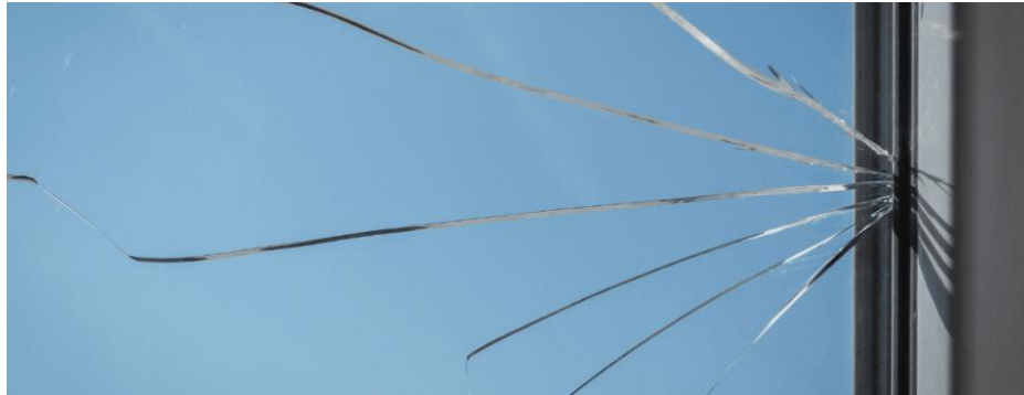
Figure 2- 23. Edge-initiated cracking pattern in monolithic glass under tensile stress.
