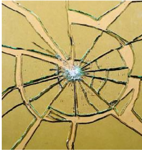
Figure 2- 15. Breakage pattern of annealed glass.
