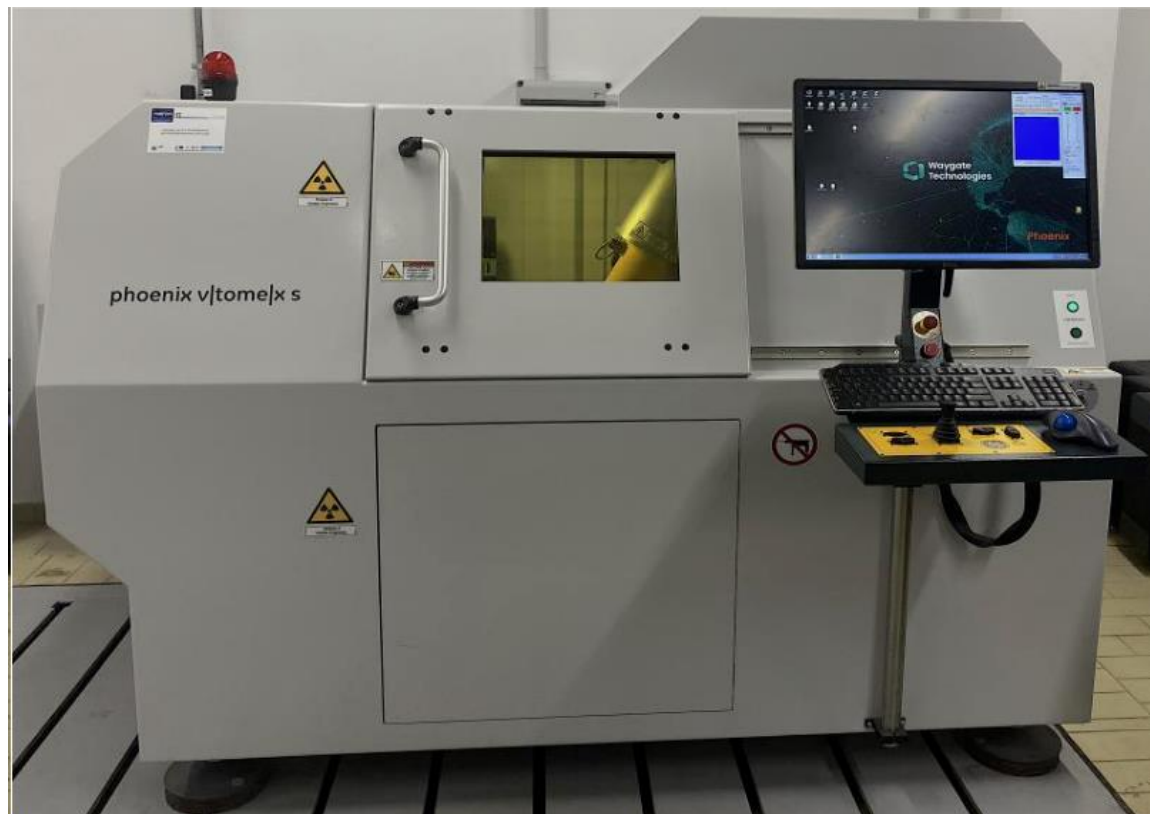
Fig 27 The X-ray computed tomography (XCT) system used for porosity analysis[201]
