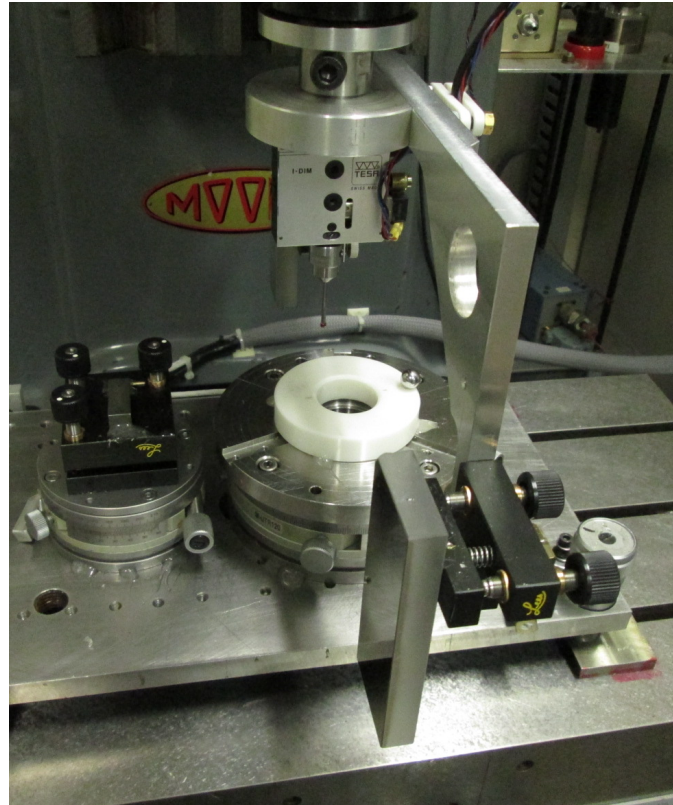
Figure 1.4: Setup for diameter measurement of a ring sample with 10 mm gauge block mounted next to the sample.
