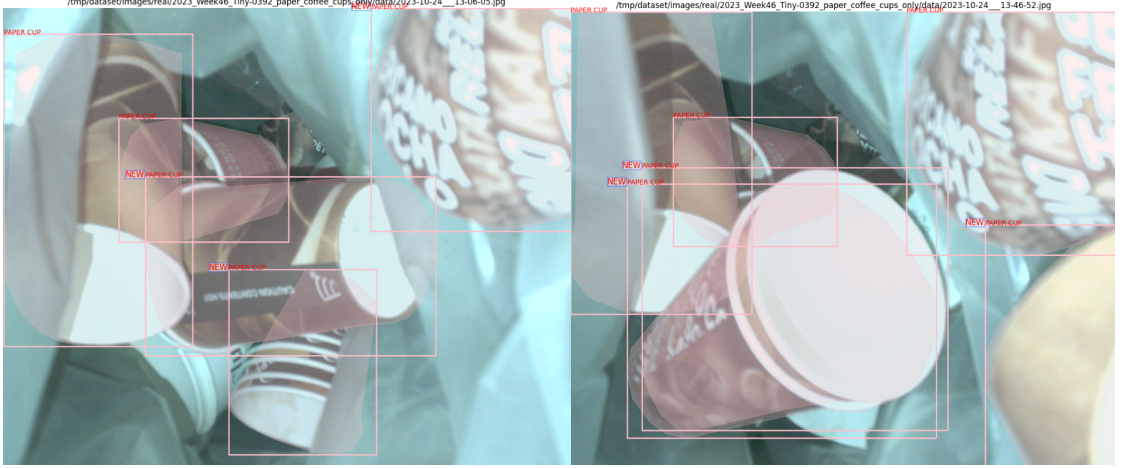
Figure 4.8: Example of a false positive for each architecture. A new object (paper cup) is mistakenly associated with a previously seen one due to strong visual similarity.
