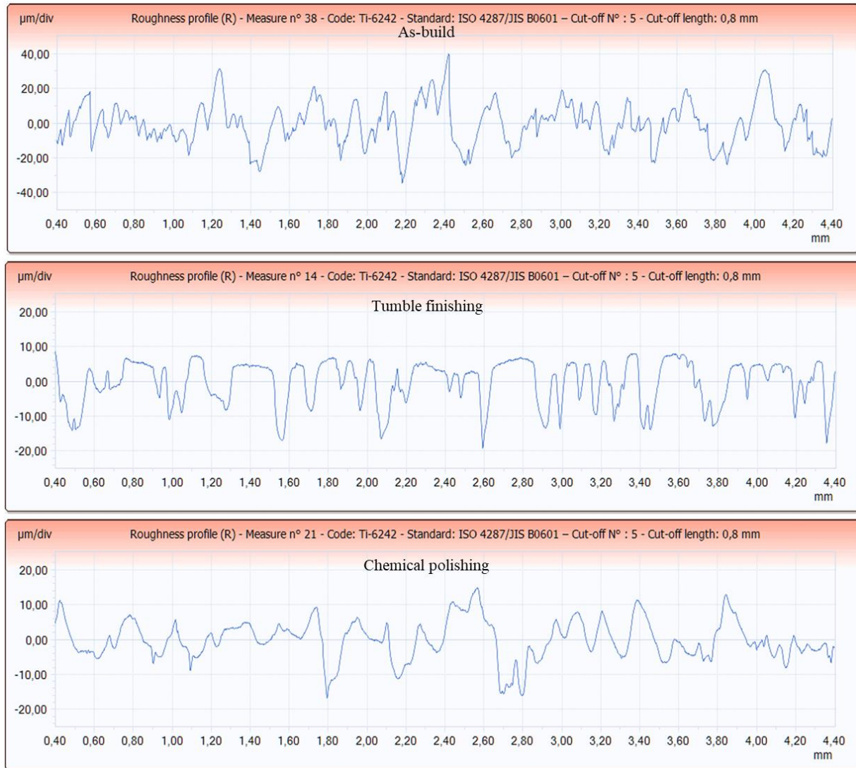
Figure 39 The roughness profile of the side walls of the parts in as-built state, tumble finished, and chemical polished
