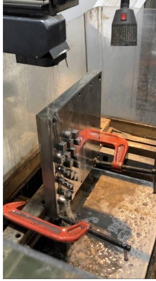
Figure 13 WEDM machine configuration during cutting
