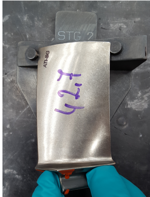
Figure 3: HPC blade measurement on the Go/NoGo tool
