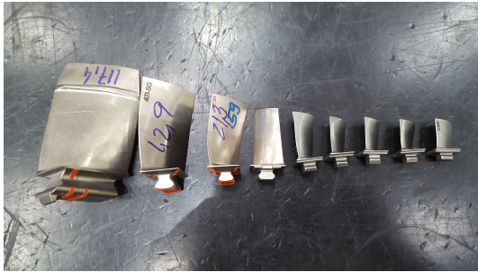
Figure 13: Blades from the CFM56-5B HPC: stage 1 to 9
