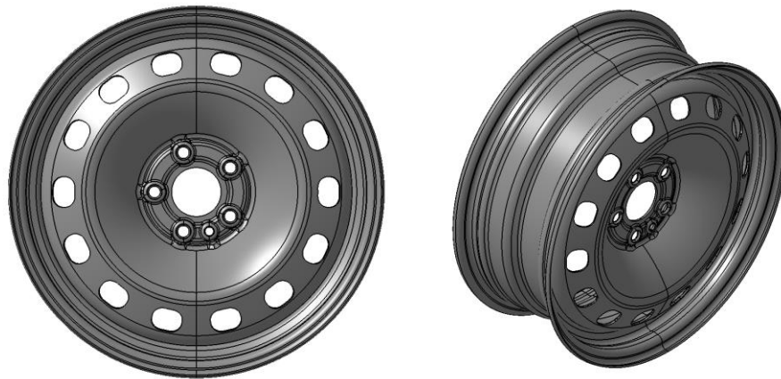
Figure 7. 0215X Automotive steel rim. Front and Isometric views.
