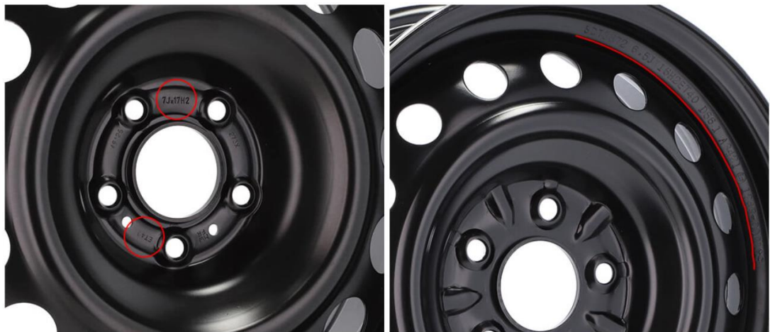
Figure 1. Identification Markings on Steel Wheel Rims
