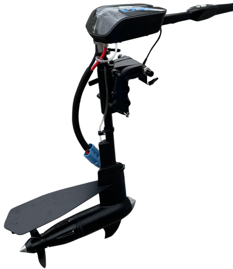
Figure 1.6. Propulsion system, 48V 10.5 kW
