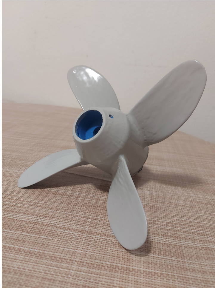
Figure 1.7. 3D printed propeller with optimized design for the endurance race.
