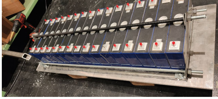
Figure 1.5. Assembling of the battery pack on the dedicated plate.
