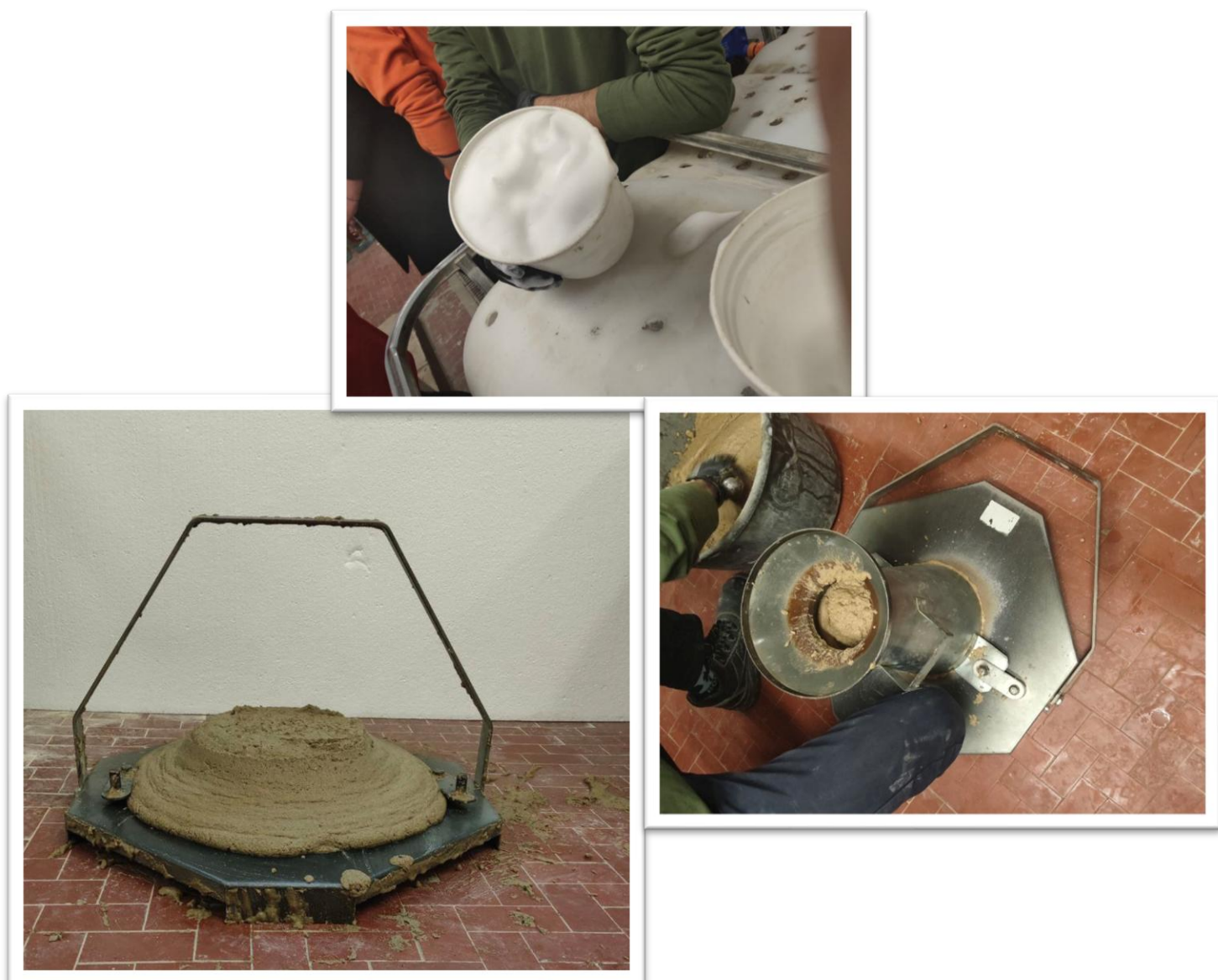
Figure 15_ The process of soil conditioning with foam to have the slump test
