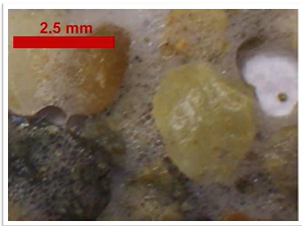
Figure10_The presence of the bubbles between the voids existed among the grains.
