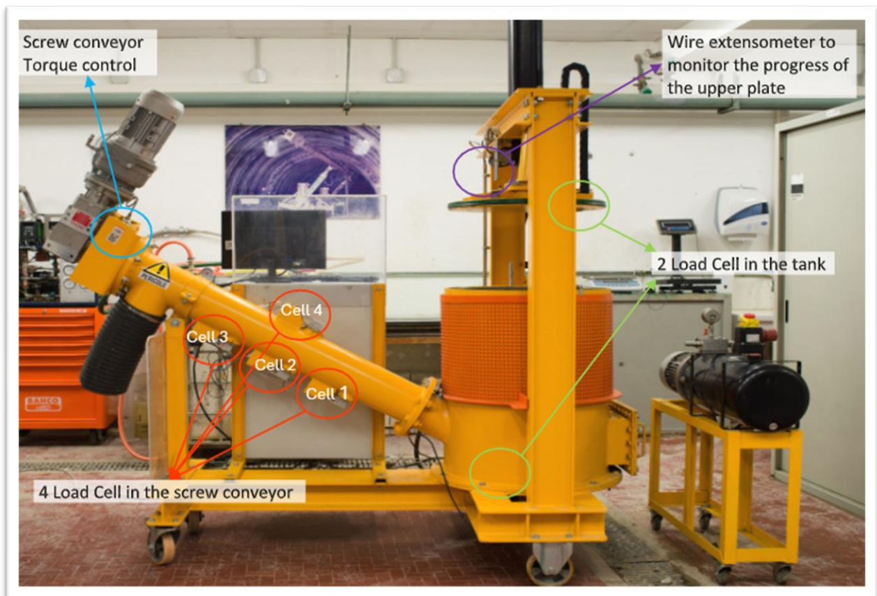
Figure 19_Screw Conveyor extraction test device.
