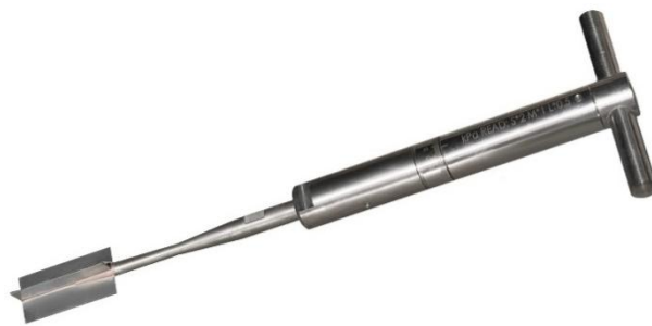
Figure 18 Modified vane test device
