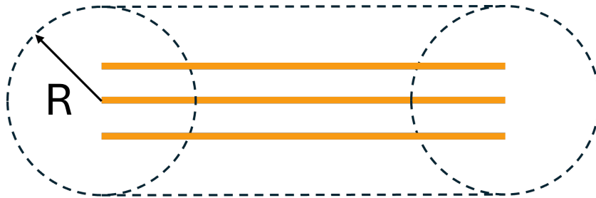
Figure 4.6: Clearance zone in the far-field approximation for a three-phase planar system
