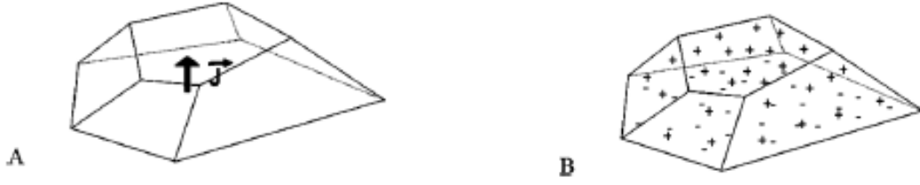
Figure 2.1: Example of polyhedron-shaped magnet. (A) Constant and uniform magnetization J [T]. (B) Equivalent Coulombian representation [2]
