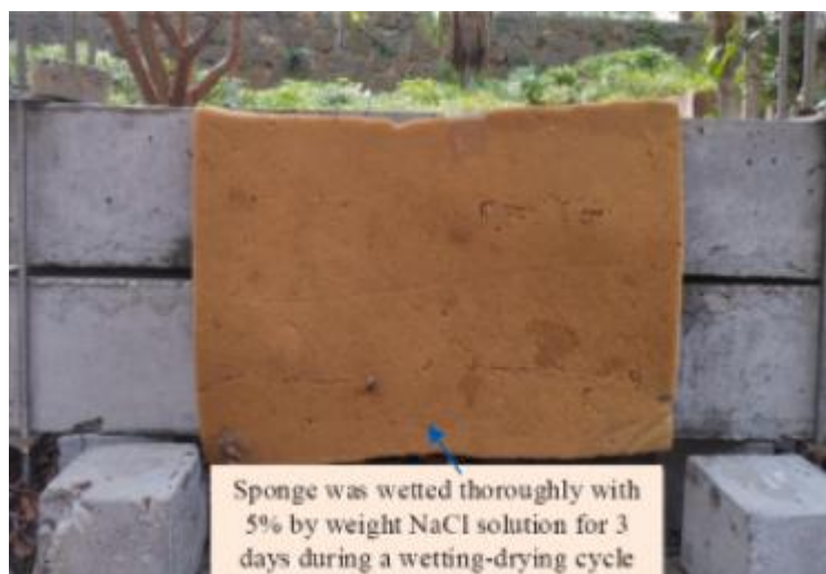
Figure 24. Chloride diffusion test with a sponge applied to the contact area [43]
