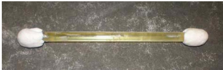
Figure 38. Glass tube filled with epoxy and sealed with aquastick [54]
