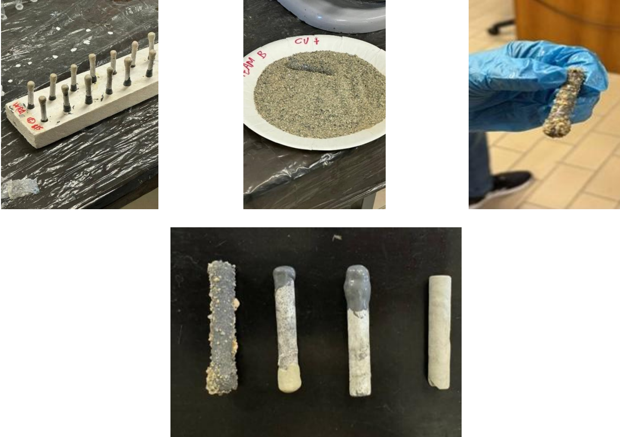
Figure 57. Capsule shell production procedures
