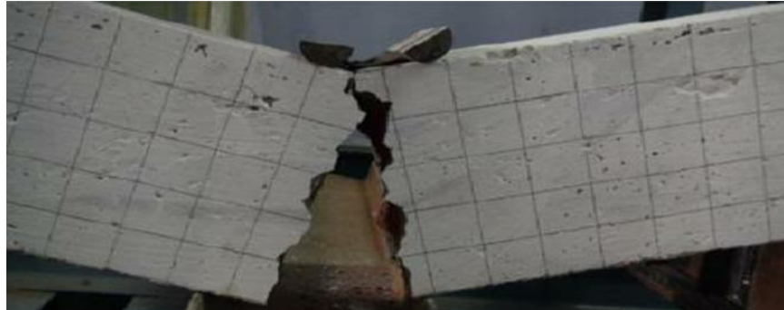
Figure 6. Flexural-brittle failure of an un-strengthened concrete beam [21]
