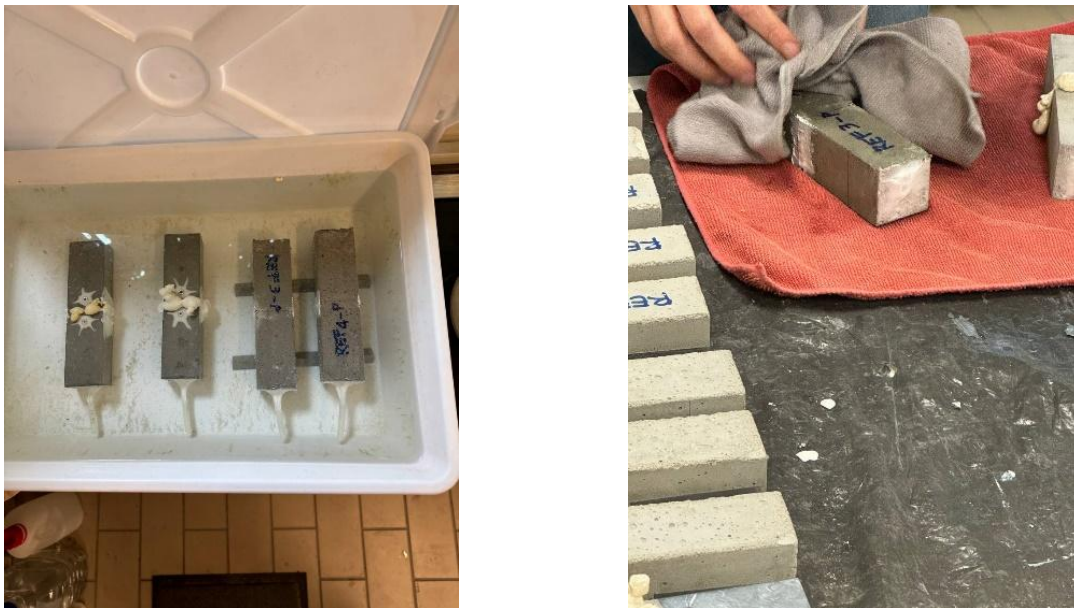
Figure 73. Submerging and surface drying of the specimens
