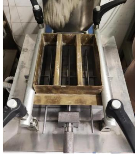
Figure 62. Casting the molds and putting on vibrating machine
