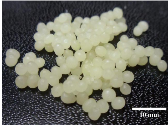
Figure 28. Calcium alginate capsules with encapsulated sunflower oil [59]
