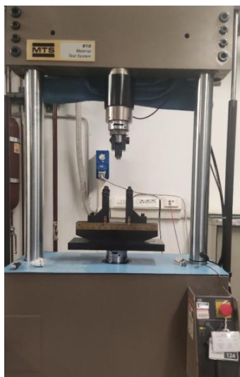
Figure 66. MTS810 servo-hydraulic press machine
