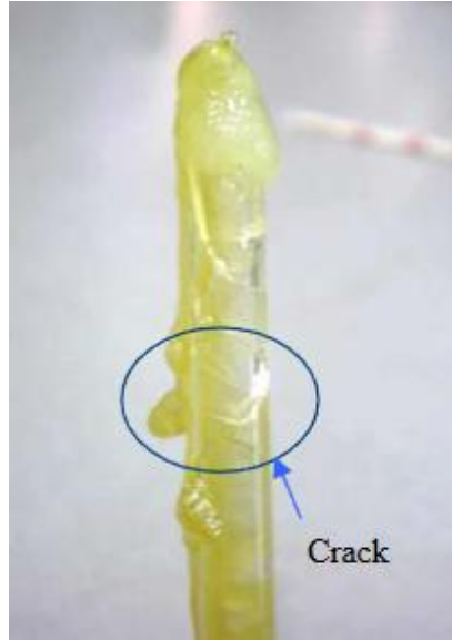
Figure 39. Perspex capsule shell filled with POR-15 epoxy, resulting in the obvious fissures [54]
