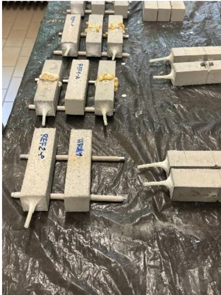
Figure 69. Foaming of Polyurethane after cracking
