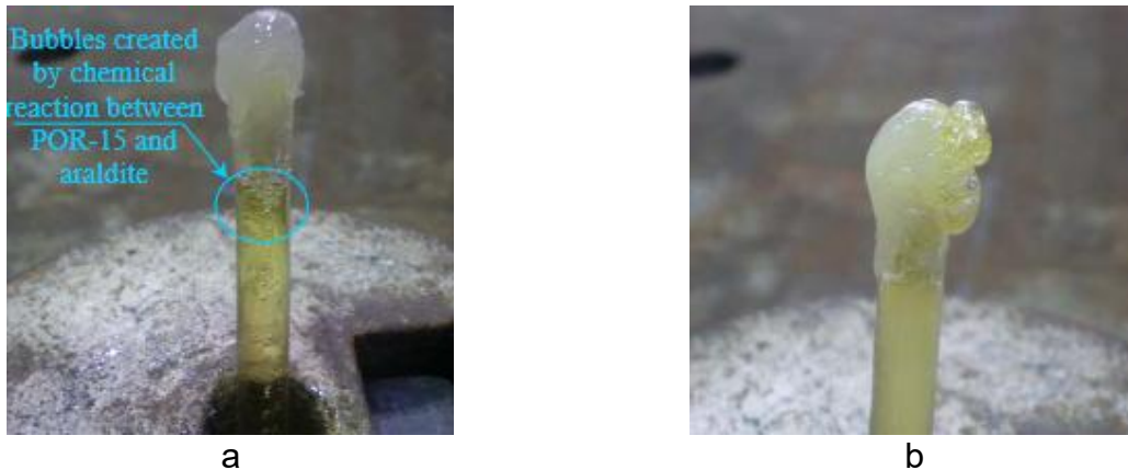
Figure 40. Epoxy leakage when araldite was used as a cap material to seal the capsules. a) after 30 minutes, and b) after 1 day sealing [54]
