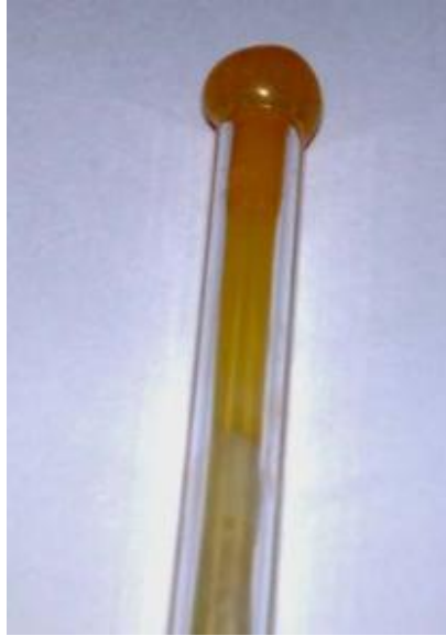
Figure 37. Glass capsule shell filled with POR-15 epoxy [54]
