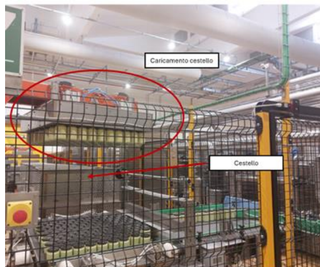
Figure 27: Autoclave basket loading process. Provided by the company
