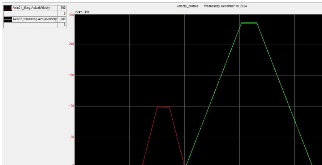
Figure 82: resulting velocity profiles from studio 5000 simulation (lifting in red and translation in green)
