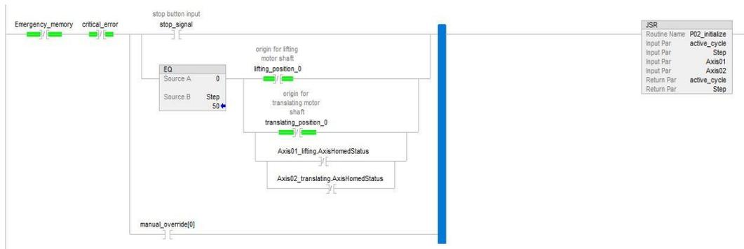
Figure 75: P02\_initialize calling rung
