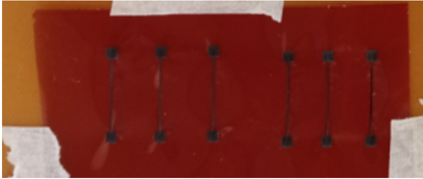
Figure 2.4: Best results: leftmost triplet: scan velocity = 350 \text{ mm s}^{-1} , rightmost triplet: scan velocity = 300 \text{ mm s}^{-1}
