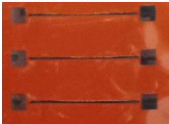
Figure 2.5: Third attempt: slightly lower homogeneity. Scan velocity = 250 \text{ mm s}^{-1}
