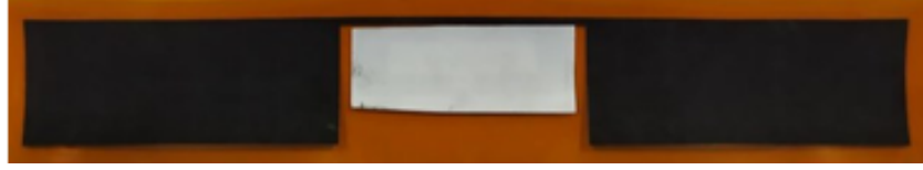
Figure 5.51: LIG on Kapton RFID: junction's length: 29.7 mm; junction's width: 0.95 mm Chietera et al. [2022]
