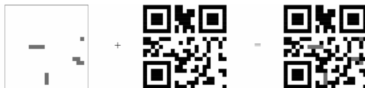
Figure 1.4: Leftmost: chromatic ink pattern; center: standard QR code; rightmost: smart QR code Fernandez et al. [2023]
