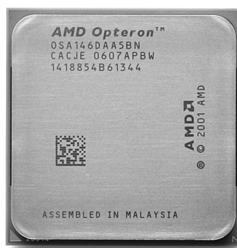
Figure 1.3: AMD Opteron the first CPU to introduce the x86-64 extensions in April 2003. ( From wikimedia.org )
