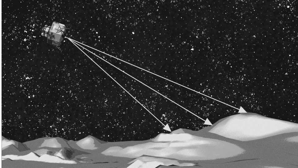
Figure 1.6: Perseverance’s AI-driven Terrain Relative Navigation (TRN) system analyzes the Martian surface to autonomously select a safe landing site. ( From nasa.com )
