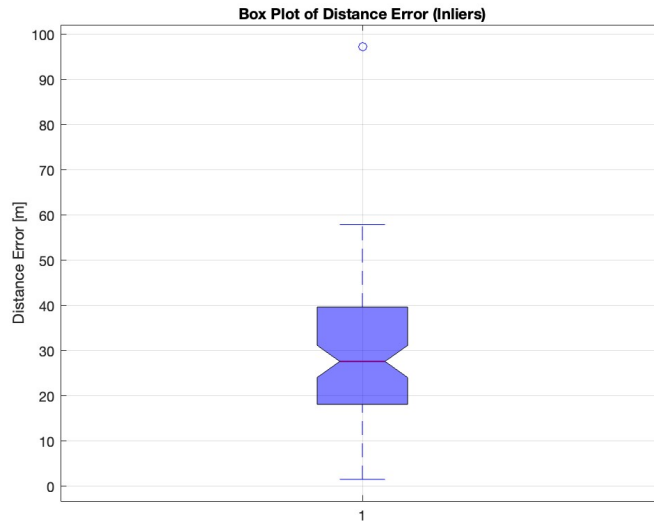
Figure 7.11: RANSAC Estimated Position Error Box-Plot
