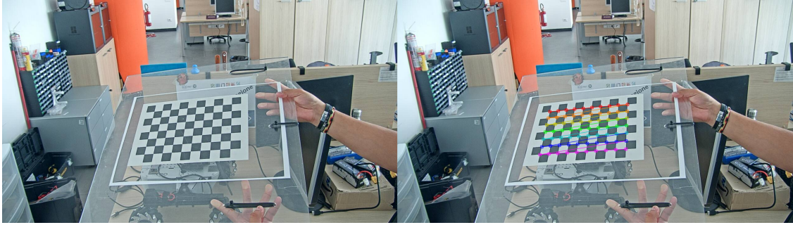
Figure 2.3. On the left the chessboard pattern used for calibration. On the right the location of 2D points.
