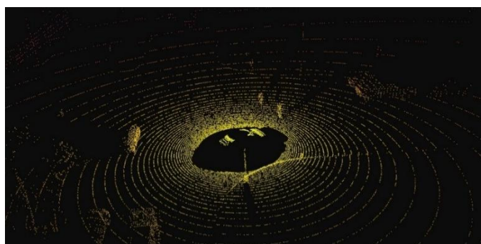
Figure 2. 2 Point cloud data of a Lidar sensor from [4].
