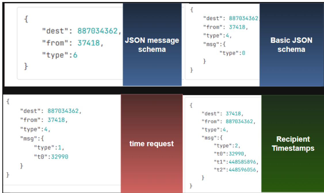
Figure 5.4. Synchronization using JSON message, reproduce from [5]
