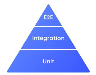
Figure 2.3. The hierarchy of testing levels
