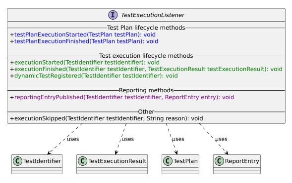
Figure 4.2. JUnit 5 TestExecutionListener Interface
