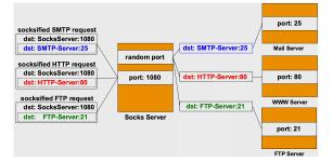
Figure 4.6. SOCKS5 Implementation Details. IP Packets are Enhanced with SOCKS5 Application-Level Data Containing Information About the Intended Destination.
