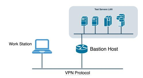
Figure 4.5. Network Layout of the Test Environment
