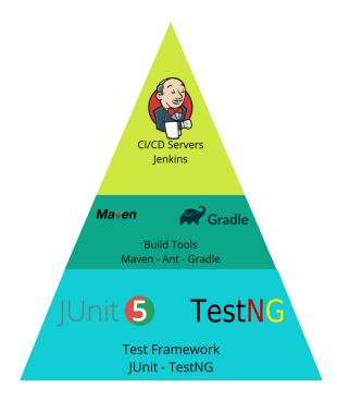
Figure 2.4. Hierarchy of the automation testing tools
