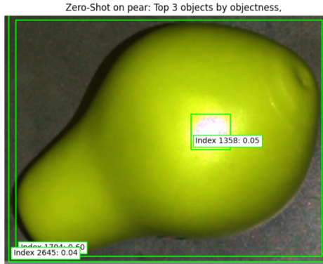
Figure 5.3: The box with maximum area has very low objectness score, while that with maximum objectness score has an area very close to the max area, so we choose the latter.
