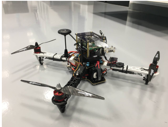
Figure 2.7: Drone Developed at CIM Using F450 Hawk's Work Frame [12].
