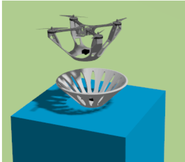
Figure 6.2: Drone and Docking Mechanism in Gazebo.
