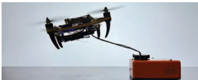
Figure 2.5: AutoCharge station connected to the drone [29].
